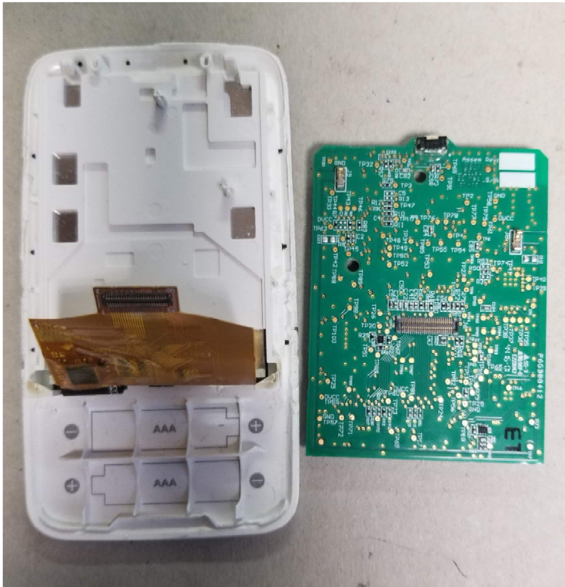
Figure 4: Front Bezel Assembly with LCD flex connector and main PCB by Side
