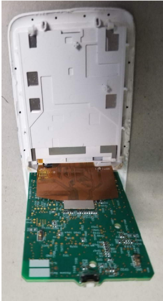
Figure 3: Main PCB lifted to display LCD assembly connector attachment on main PCB
