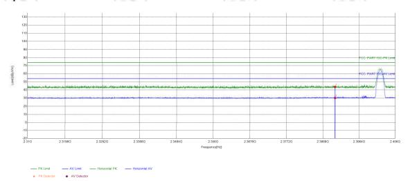
**Suspected List** Factor Limit Reading Level Margin Freq. [dB] NO Result **Polarity** Remark [MHz] [dBµV]  $[dB\mu V/m]$  $[dB\mu V/m]$ [dB] 1 2390 5.77 37.93 43.70 74.00 30.30 **PASS** Horizontal PΚ 2 2390 5.77 24.44 30.21 54.00 23.79 **PASS** Horizontal ΑV
