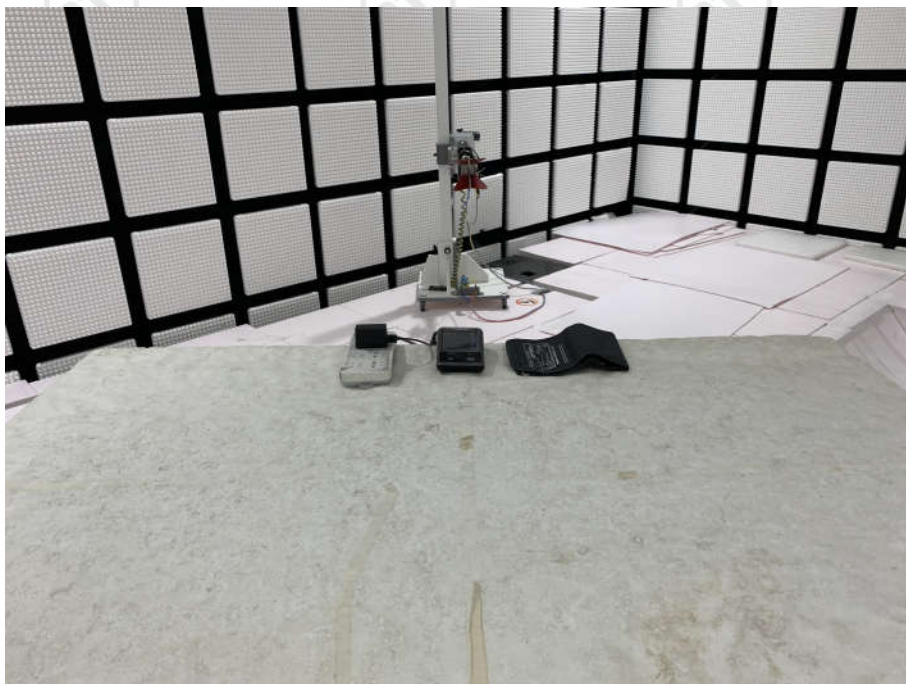
Radiated spurious emission Test Setup-2(Above 1GHz)
