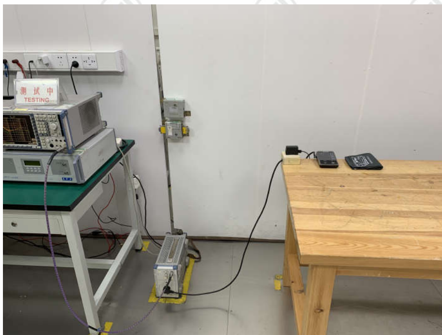
Conducted Emissions Test Setup
