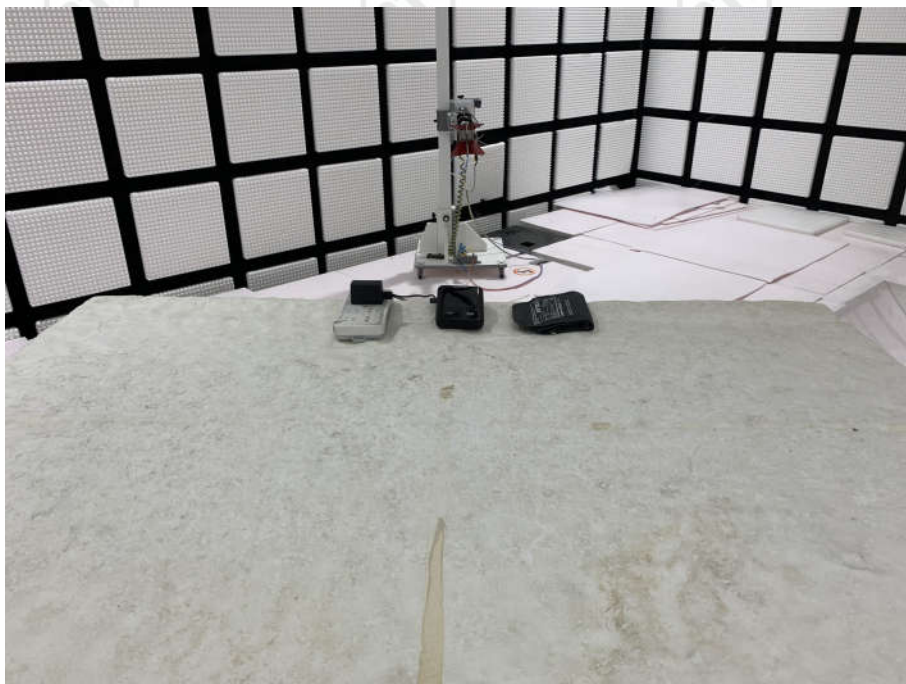
Radiated spurious emission Test Setup-2(Above 1GHz)
