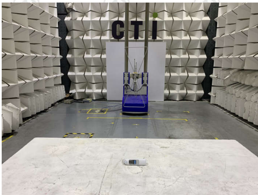
Radiated spurious emission Test Setup-1(Below 1GHz)
