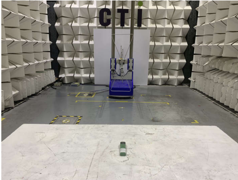
Radiated spurious emission Test Setup-1(Below 1GHz)
