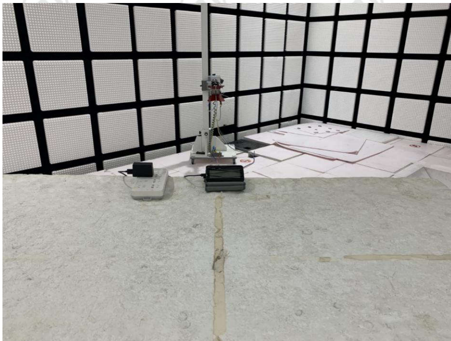
Radiated spurious emission Test Setup-2(Above 1GHz)
