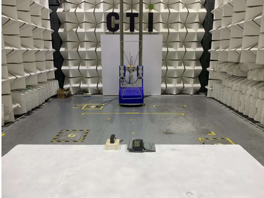
Radiated spurious emission Test Setup-1(Below 1GHz)
