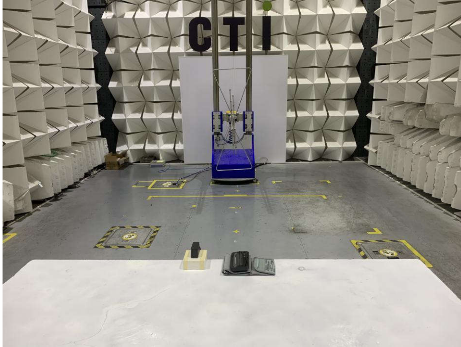
Radiated spurious emission Test Setup-1(Below 1GHz)
