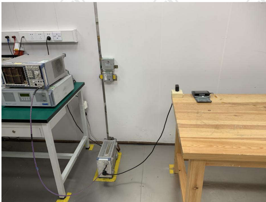
CONDUCTED EMISSION TEST SETUP
