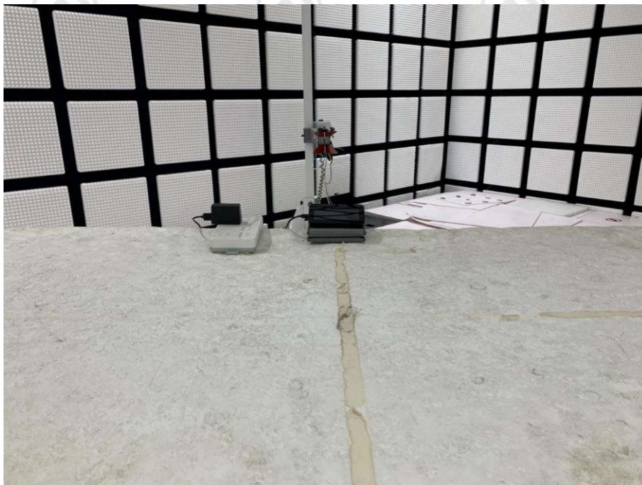
Radiated spurious emission Test Setup-2(Above 1GHz)
