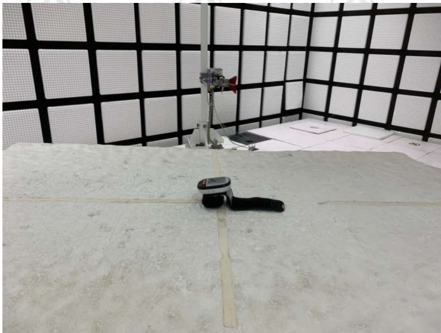
Radiated spurious emission Test Setup-2(Above 1GHz)
