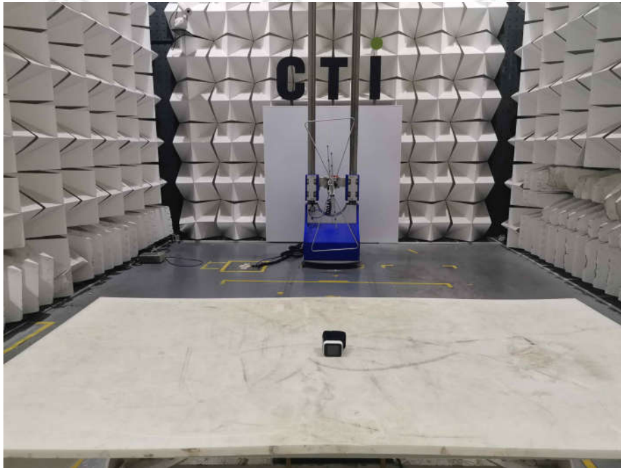
Radiated spurious emission Test Setup-1(Below 1GHz)
