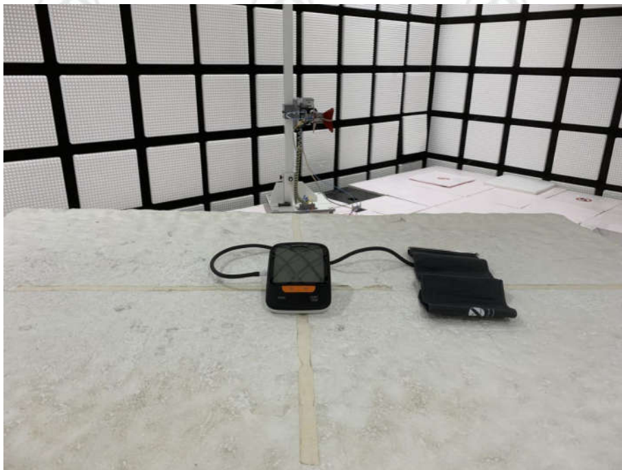
Radiated spurious emission Test Setup-2(Above 1GHz)
