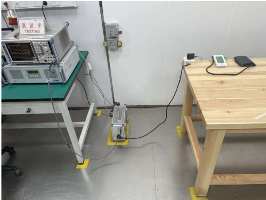
Conducted Emissions Test Setup
