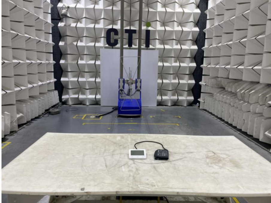
Radiated spurious emission Test Setup-1(Below 1GHz)
