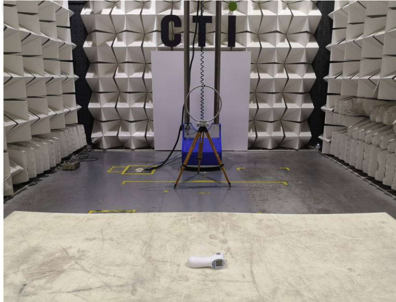
Radiated spurious emission Test Setup-1(Below 30MHz)
