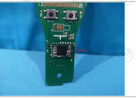
The antenna is integral antenna. The best case gain of the antenna is 0dBi.
