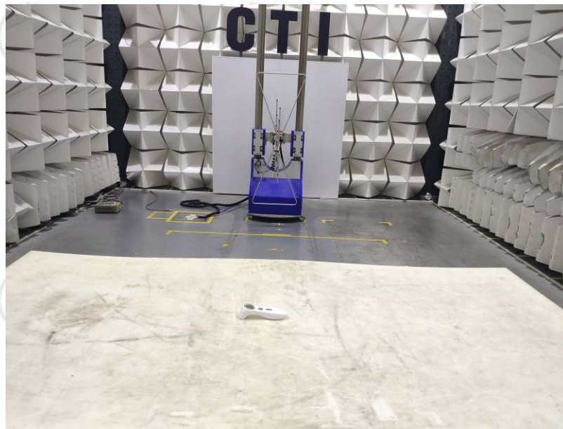
Radiated spurious emission Test Setup-2(Below 1GHz)
