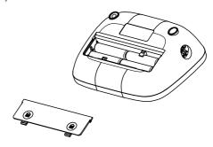
AC Adapter jack is on the right side of the monitor. Medical AC adapter (DC 6.0 V,600mA) can be used with the device (recommended, not provided). The adapter connect pin should be positive inside and negative outside with a 2.1mm coaxial joint.
