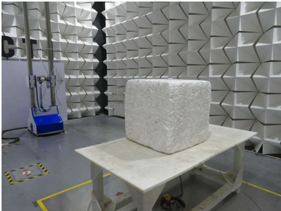
Radiated spurious emission Test Setup-2(30MHz-1GHz)
