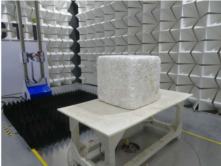
Radiated spurious emission Test Setup-3(Above 1GHz)
