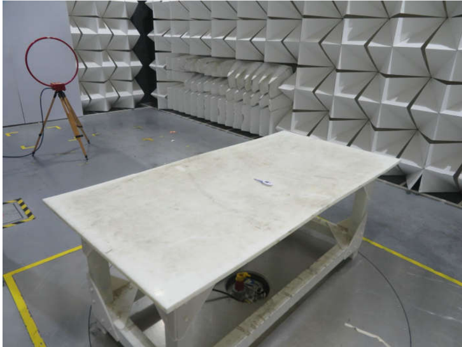
Radiated spurious emission Test Setup-1(Below 30MHz)
