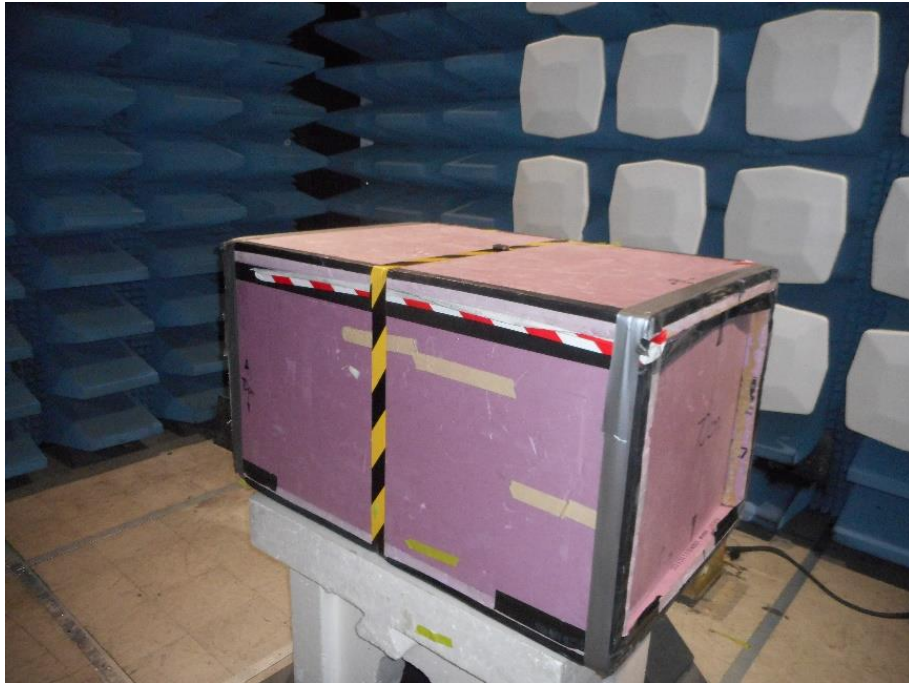
The setup of the EUT at the 3m SAC, above 1 GHz
