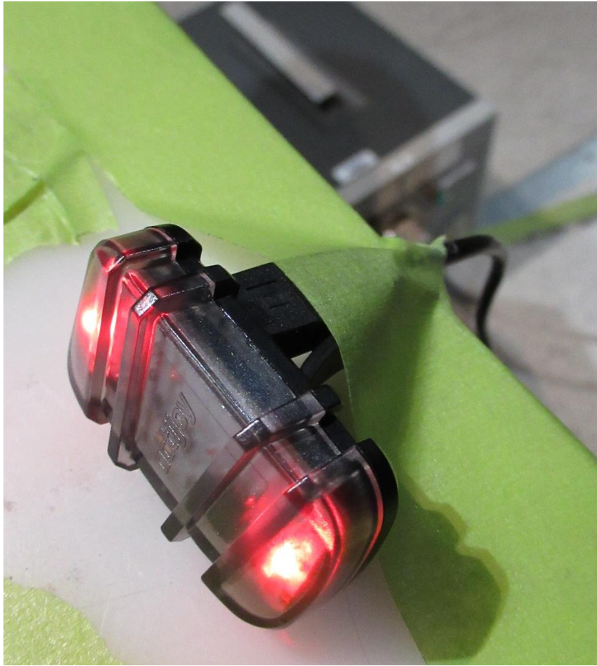
Conducted Emissions (close-up) performed at the 3m SAC
