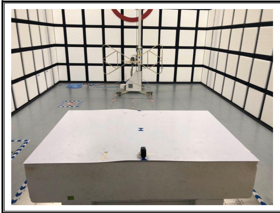
RADIATED RF MEASUREMENT SETUP (Below 30MHz)
