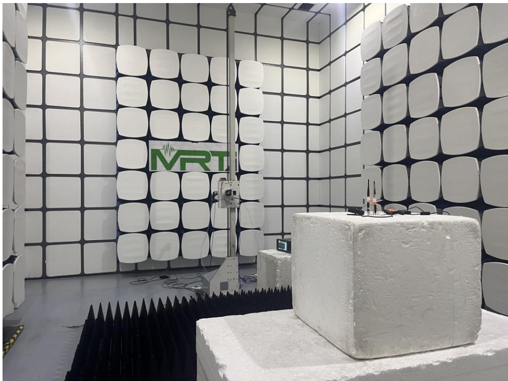
Description: Radiated Spurious Emissions Test Setup for above 18GHz
