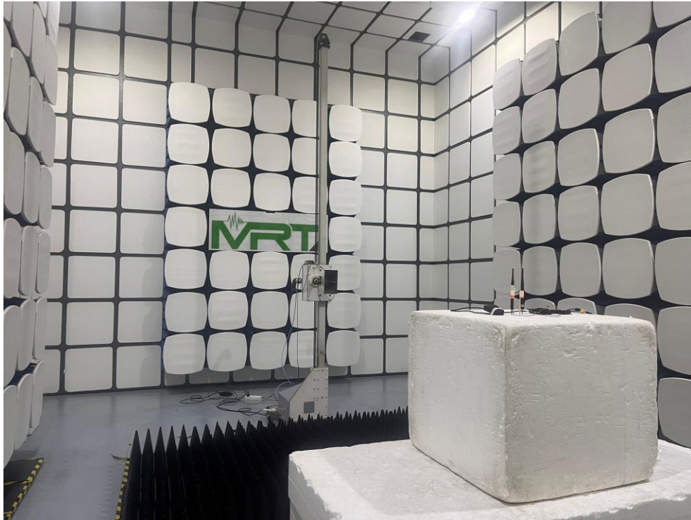
Description: Radiated Spurious Emissions Test Setup for above 18GHz
