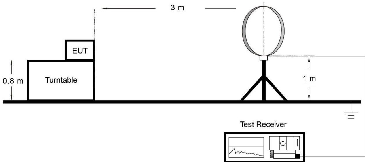
Below 1GHz Test Setup:
