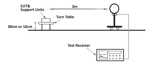
For Radiated emission 30MHz to 1GHz:
