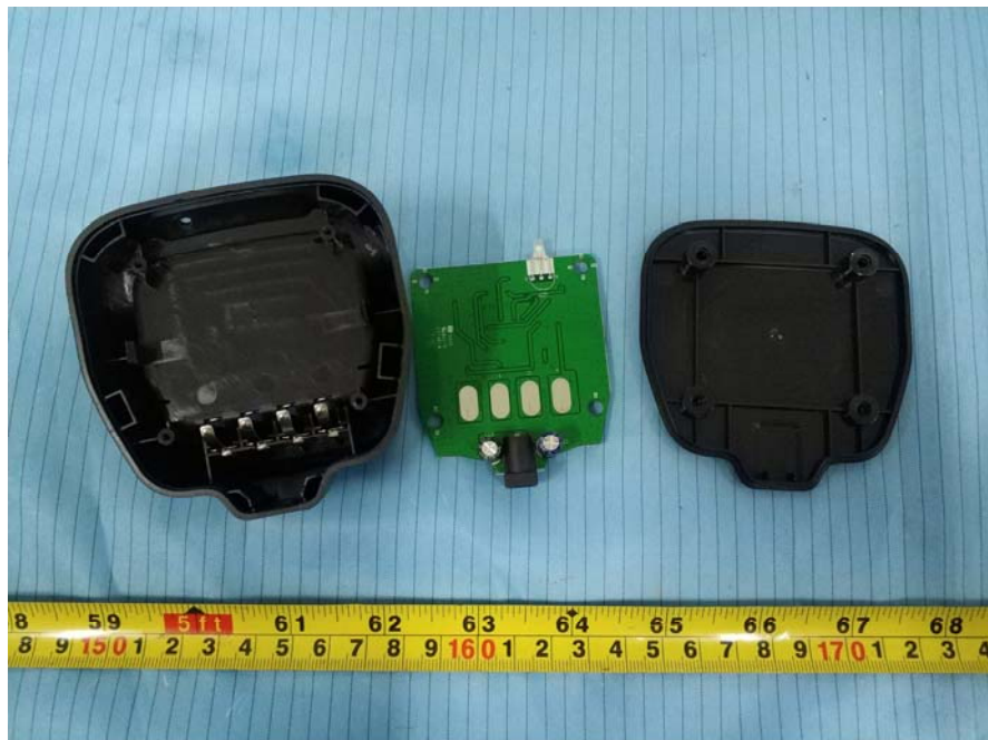
EUT (Charger) – Cover off View
