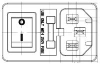
Press I to power on the AC power.Press O to power off the AC power.
