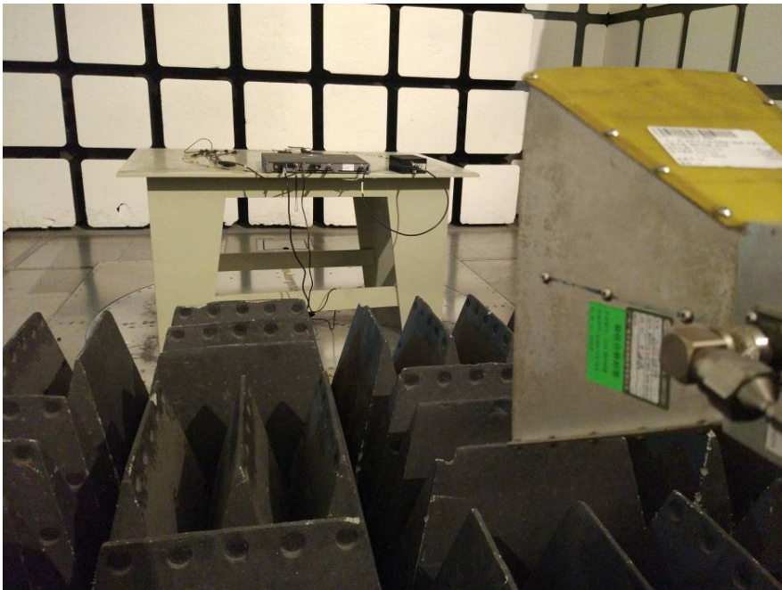
Radiated Emissions – Rear View (Above 1 GHz)
