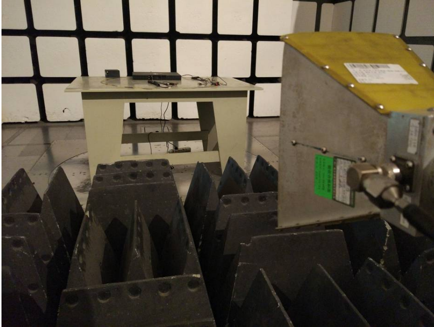
Radiated Emissions – Front View (Above 1 GHz)
