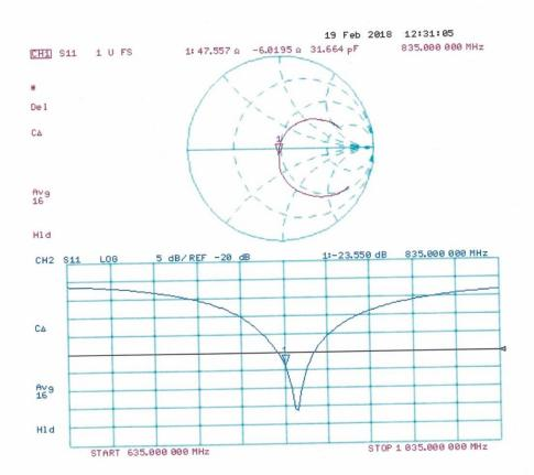
Impedance Measurement Plot for Body TSL
