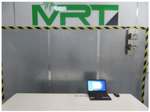
Test Mode 1 Description: Side View of Conducted Emission Test Setup
