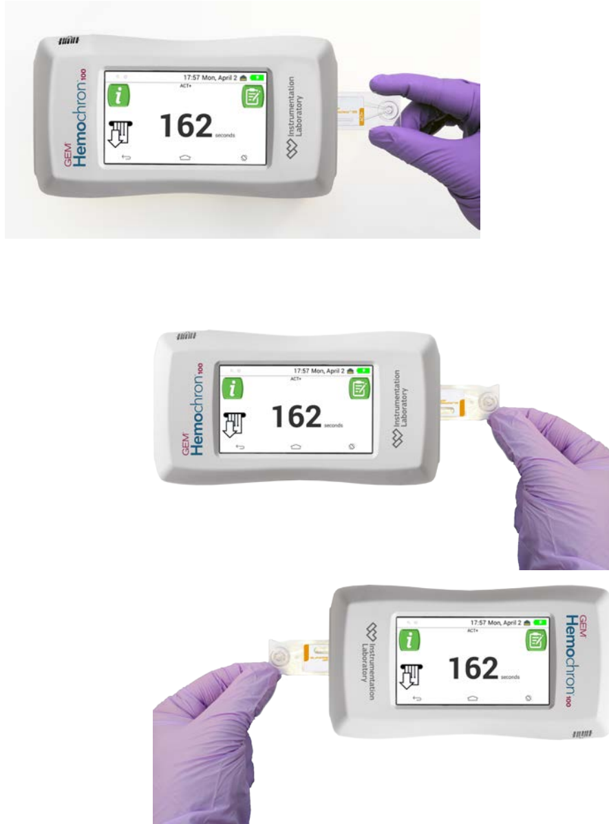
Figure 10 – The Rotate Screen icon allows for instrument use with the cuvette slot on the left end or right end
