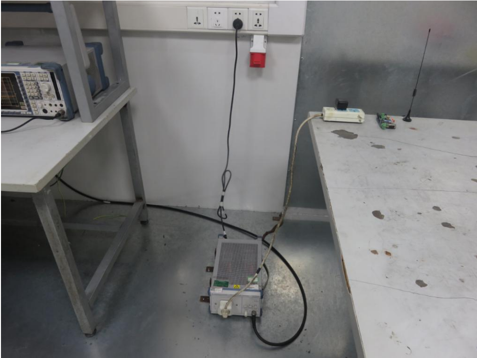
Photo of Power Line Conducted Emission Test
