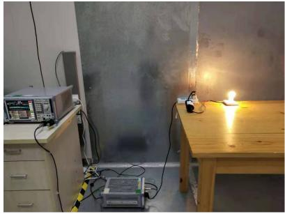
Radiated Spurious Emissions Test Frequency From 30MHz-1000MHz
