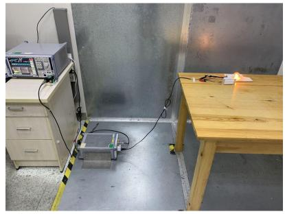
Radiated Spurious Emissions From 30MHz-1000MHz
