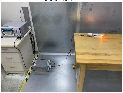
Radiated Spurious Emissions From 30MHz-1000MHz
