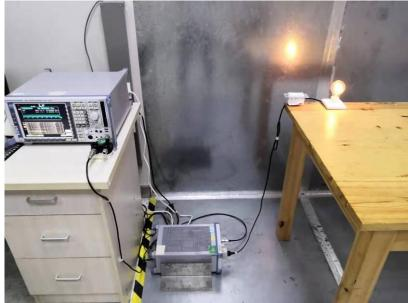
Radiated Spurious Emissions Test Frequency From 30MHz-1000MHz
