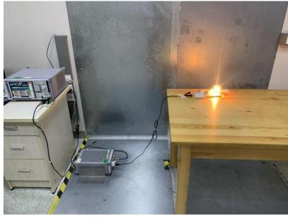
Radiated Spurious Emissions From 30MHz-1000MHz
