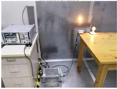
Radiated Spurious Emissions Test Frequency From 30MHz-1000MHz
