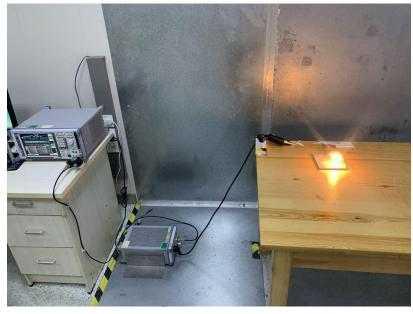
Radiated Spurious Emissions From 30MHz-1000MHz
