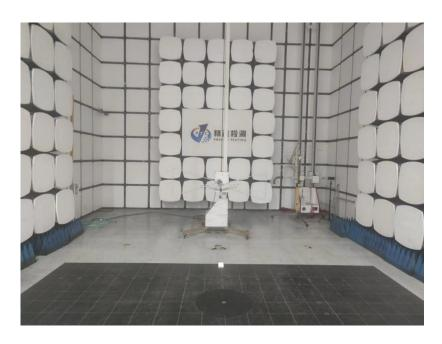
Radiated Emissions From 30MHz-1000MHz
