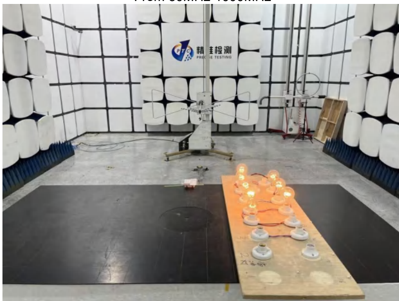
Radiated Spurious Emissions From 30MHz-1000MHz
