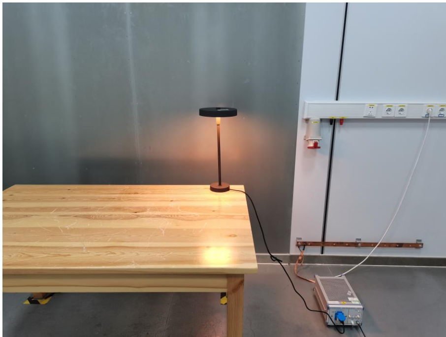
Fig. 4 Power line conducted emission setup photo
