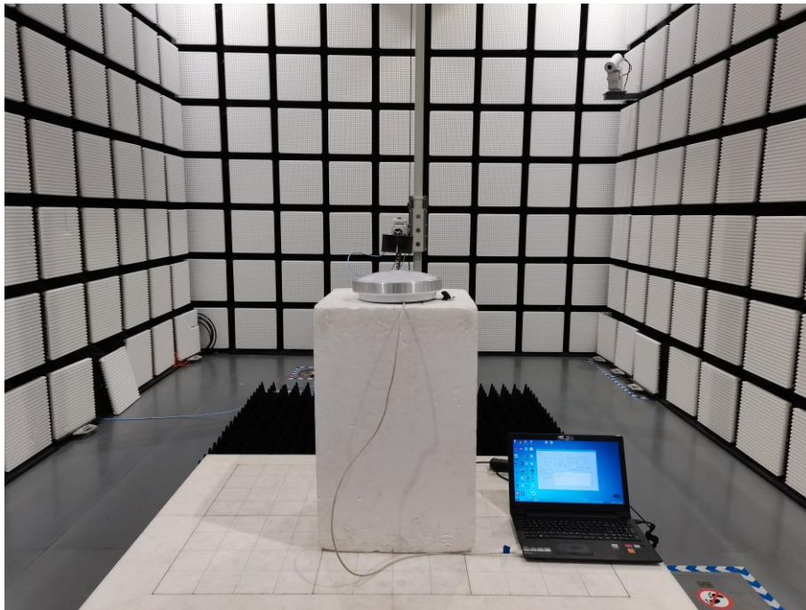
Fig. 3 Radiated emission setup photo(Above 1GHz)
