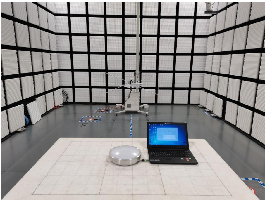
Fig. 2 Radiated emission setup photo(30MHz-1GHz)
