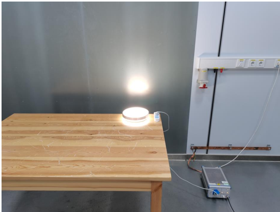
Fig. 4 Power line conducted emission setup photo
