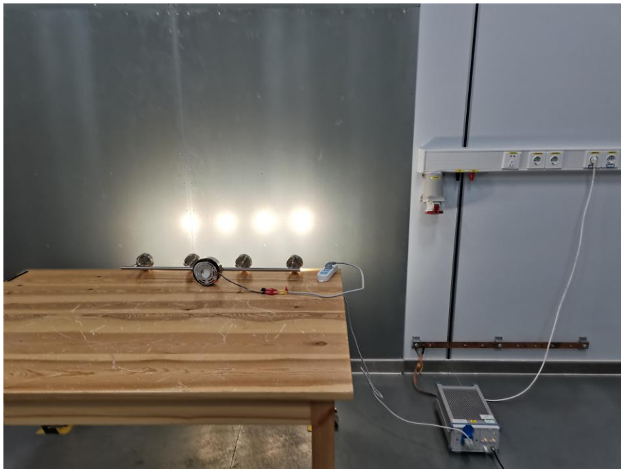
Fig. 4 Power line conducted emission setup photo
