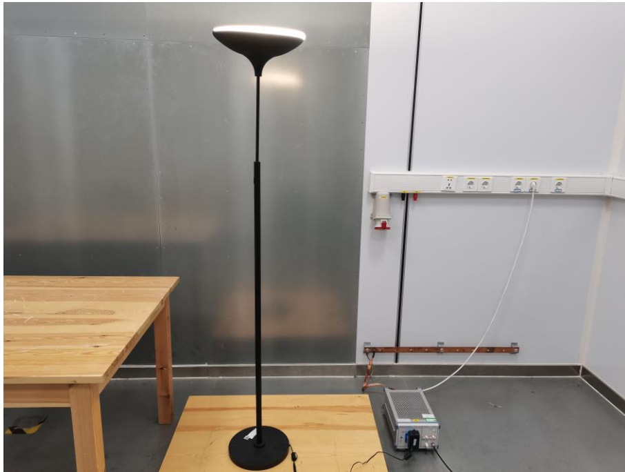
Fig. 4 Power line conducted emission setup photo
