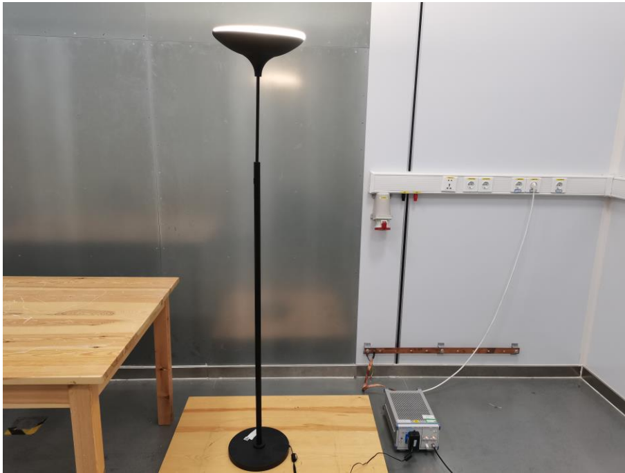
Fig. 4 Power line conducted emission setup photo
