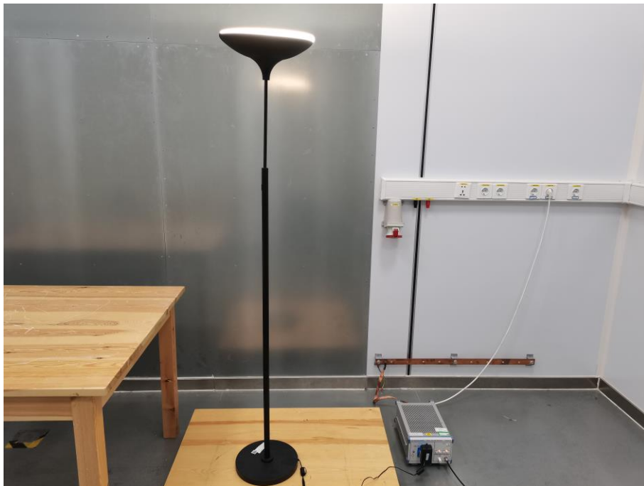
Fig. 4 Power line conducted emission setup photo
