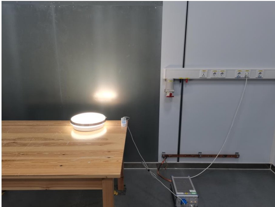
Fig. 4 Power line conducted emission setup photo
