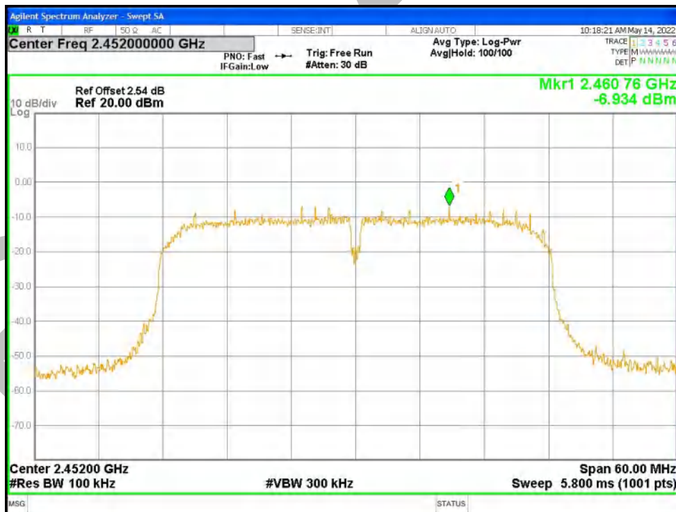
Tx. Spurious NVNT n40 2452MHz Ant1 Emission
