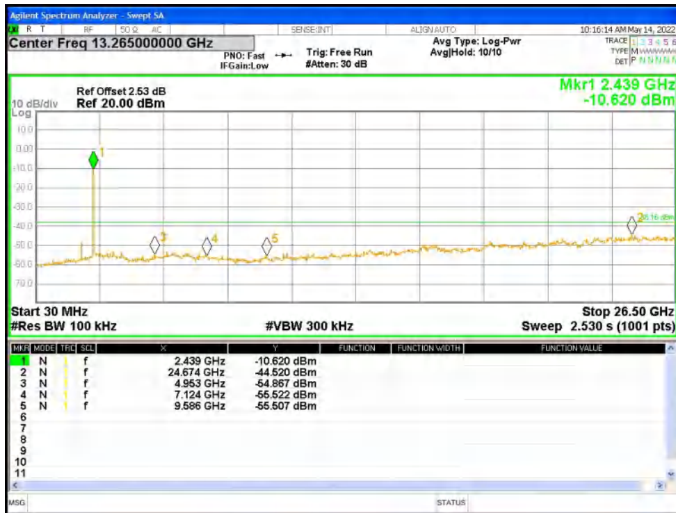
Tx. Spurious NVNT n40 2452MHz Ant1 Ref
