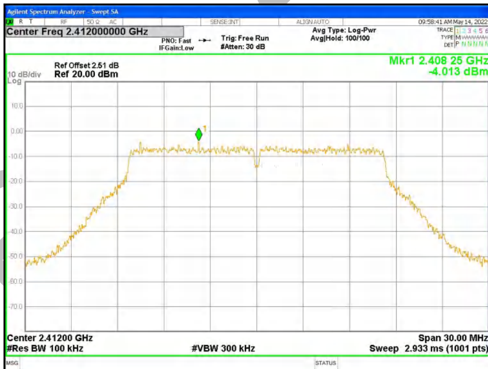
Tx. Spurious NVNT g 2412MHz Ant1 Emission
