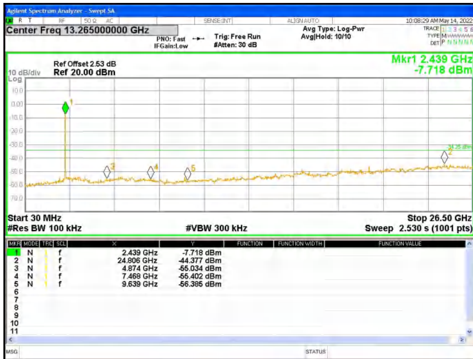
Tx. Spurious NVNT n20 2462MHz Ant1 Ref
