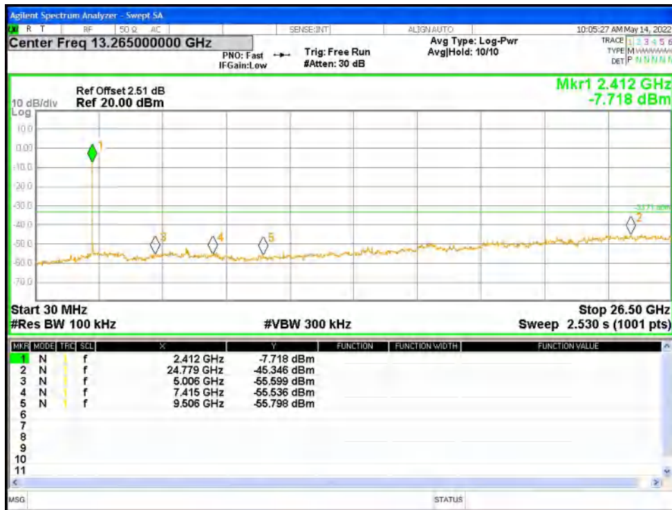
Tx. Spurious NVNT n20 2437MHz Ant1 Ref
