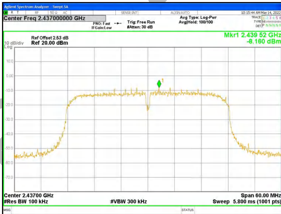
Tx. Spurious NVNT n40 2437MHz Ant1 Emission
