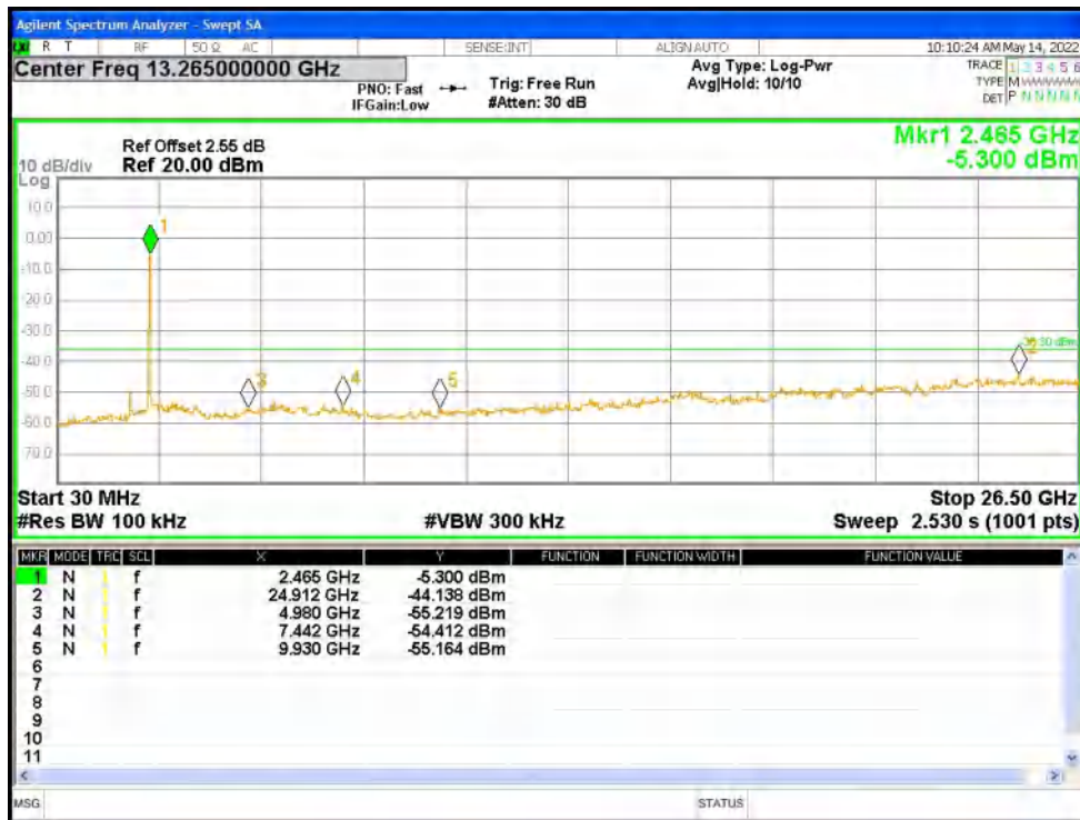
Tx. Spurious NVNT n40 2422MHz Ant1 Ref
