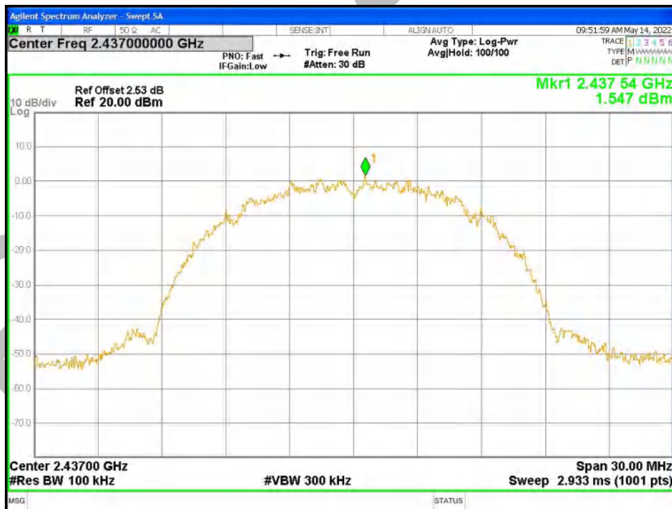
Tx. Spurious NVNT b 2437MHz Ant1 Emission
