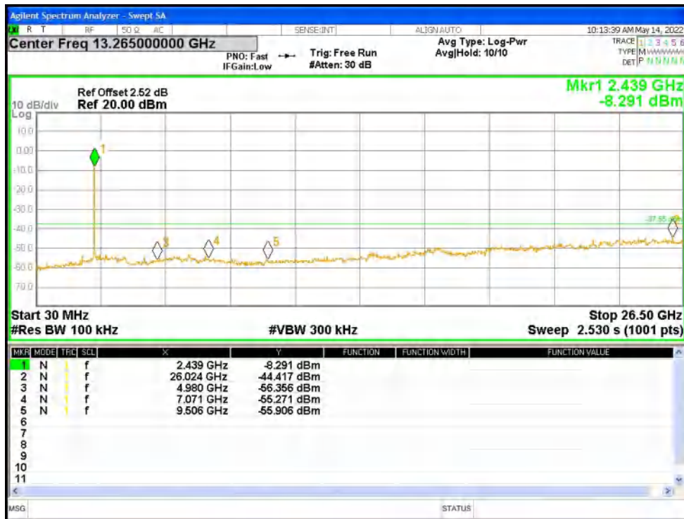
Tx. Spurious NVNT n40 2437MHz Ant1 Ref
