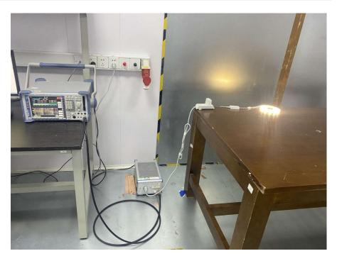
Conducted Emissions at Mains Terminals (150kHz-30MHz)
