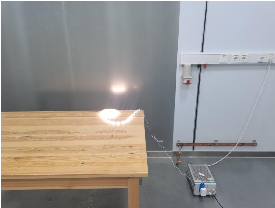
Fig. 4 Power line conducted emission setup photo
