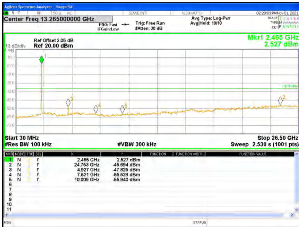
Tx. Spurious NVNT g 2412MHz Ant1 Ref
