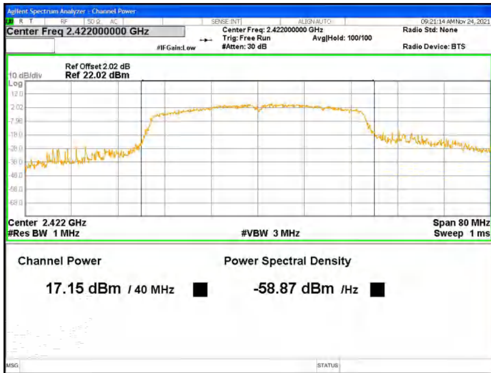
Power NVNT n40 2437MHz Ant1
