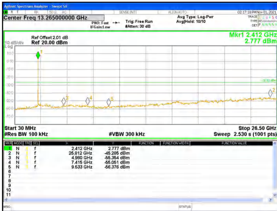
Tx. Spurious NVNT b 2437MHz Ant1 Ref
