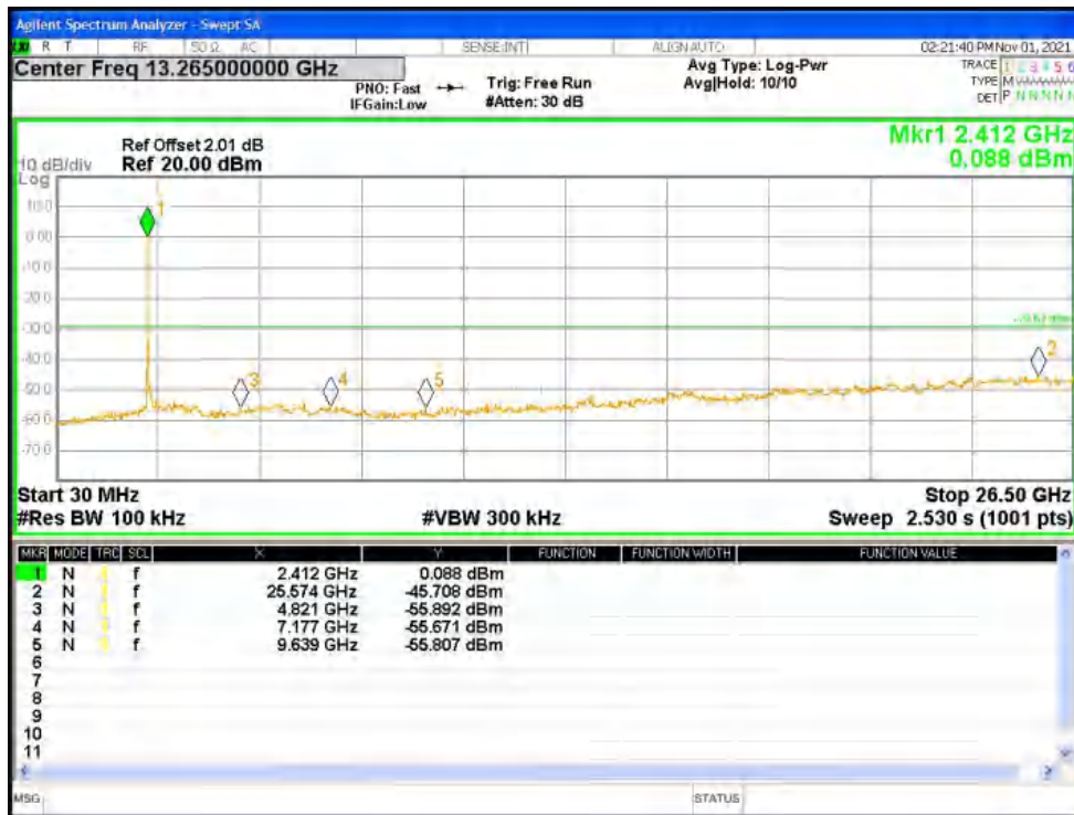
Tx. Spurious NVNT g 2437MHz Ant1 Ref
