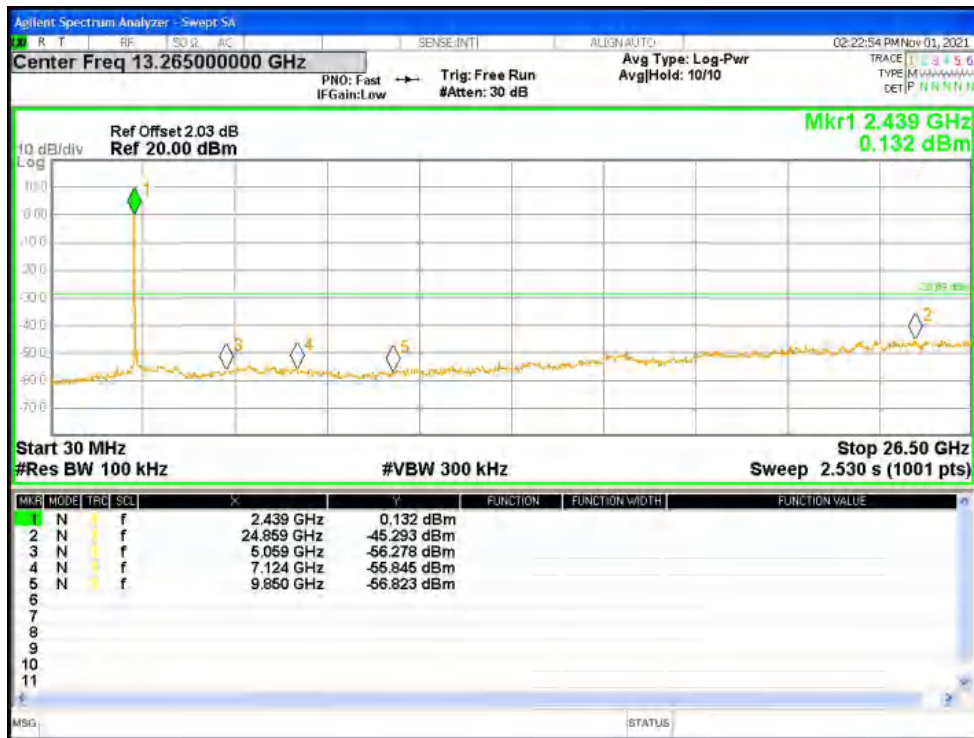
Tx. Spurious NVNT g 2462MHz Ant1 Ref
