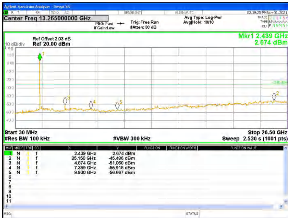
Tx. Spurious NVNT b 2462MHz Ant1 Ref
